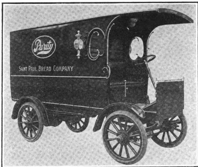
Purity Electric truck with two-speed sliding gearset
